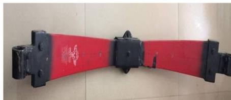
Fig 2 Composite mono leaf spring
