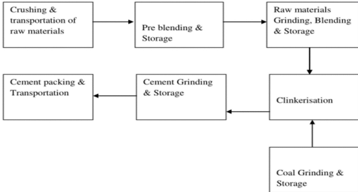
Fig.2 Block diagram of Cement making Process
