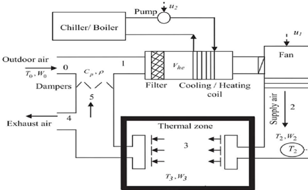
Fig.3 Block diagram of air conditioner system using VFD
