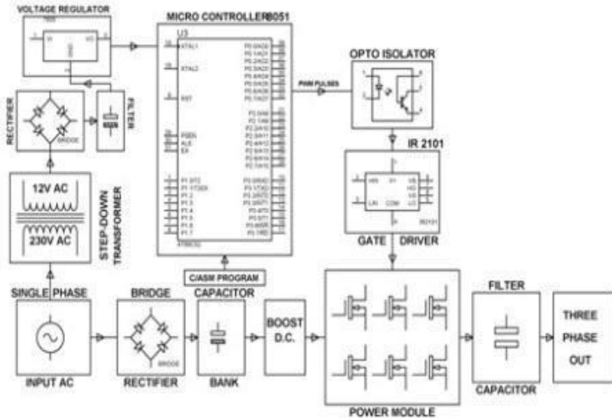
Fig. Variable Frequency Drive
