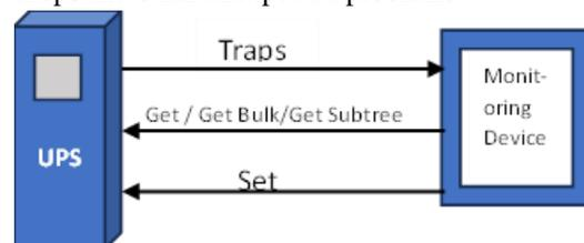
Figure 2: Primary functions to exchange data between UPS and Monitoring Device
