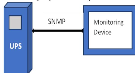
Figure 1: Data exchange between UPS and Monitoring Device using SNMP Protocol
