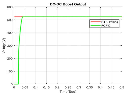
Figure 5:DC-DC Boost Output for Voltage
