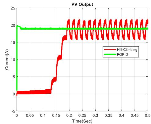
Figure 3: PV output for Current v/s time
