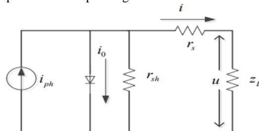
Fig.1 physical model of photovoltaic cell [4]
