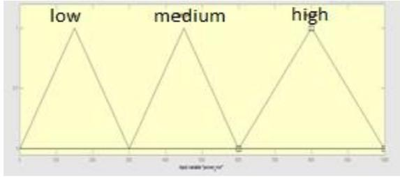
Fig. 4: Membership function for power error.
