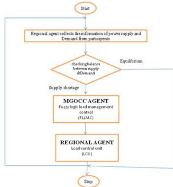
Fig. 9: Flow Chart of Load Shedding System.
