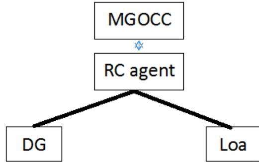
Fig. 6: Basic Structure of a MAS for Islanded Microgrid Operation.
