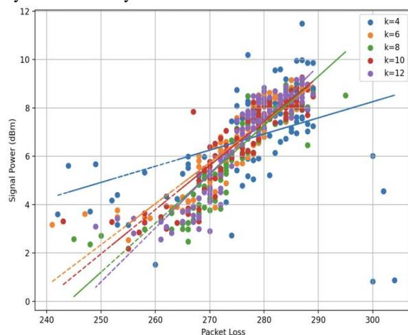
Figure 5: Packet Loss Variation w.r.t Signal Power during Downlink Communication
