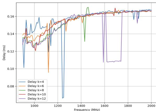
Figure 6: Transmission Delay variation w.r.t Frequency
