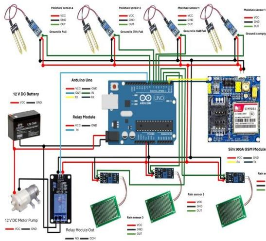
Powering the system is facilitated by the battery, with its positive terminal connected to the Arduino's voltage input pin. This provides power to the Arduino and other components, ensuring uninterrupted operation. Ground connections complete the circuit, ensuring stable power distribution throughout the system.
