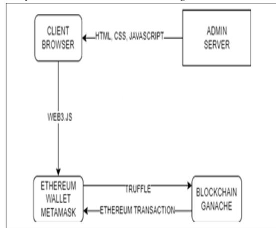
Fig. 1. Architecture of the system
