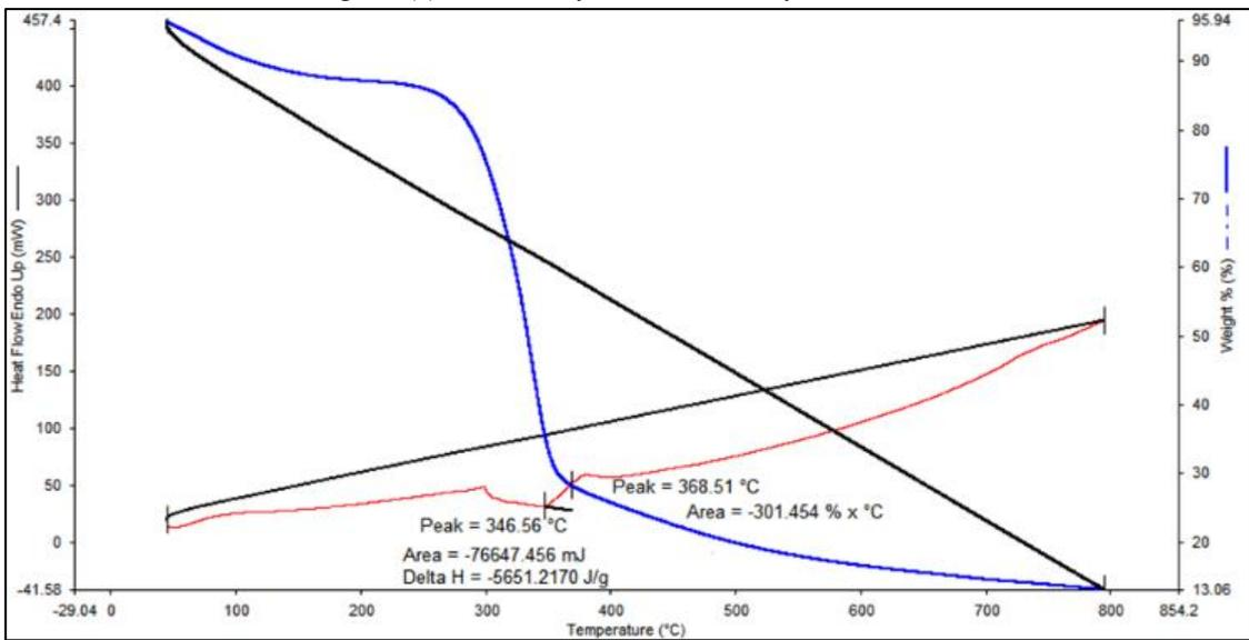
Fig. 10 (b). TGA Analysis of Treated Paddy Straw Fiber
