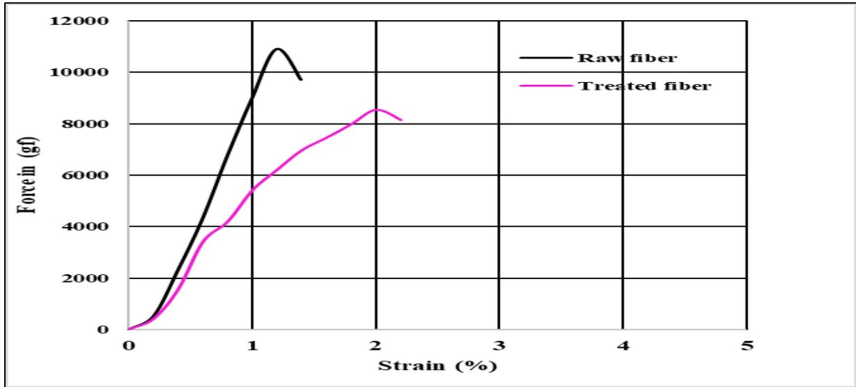
Fig. 7. Single Fiber Test – Raw and Treated Fiber
