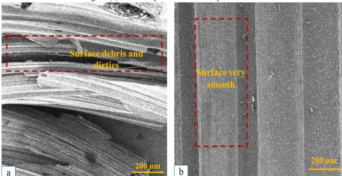
Fig. 11. SEM Micrograph of Raw and Treated Fiber Composites
