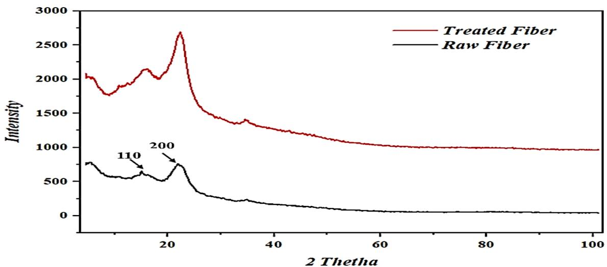
Fig. 8. X-ray diffraction Analysis of Paddy Straw Fiber
