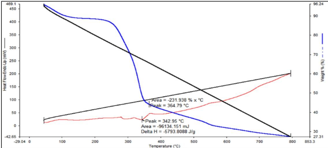
Fig. 10 (a). TGA Analysis of Raw Paddy Straw Fiber
