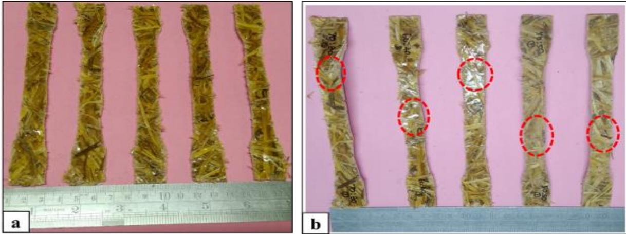
Fig. 2. Tensile Test Fractured Specimens A) Before B) After
