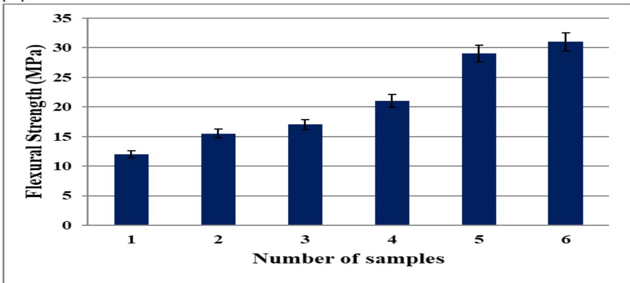
Fig. 4. Flexural Strength for Different Composite (paddy straw)
