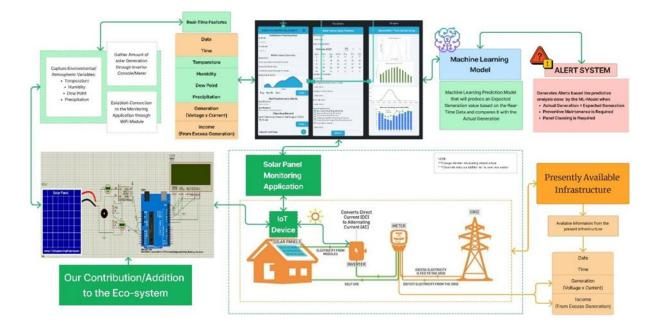
The IoT device with the sensor was placed directly alongside the solar panels, providing real-time data that could be fed into the analysis pipeline for energy forecasting and cleaning optimization. The infrastructure was designed to be scalable, with the potential to incorporate additional sensors in the future, such as dust and particulate matter sensors.
