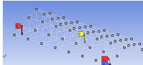
Figure 4: Loads and boundary conditions
