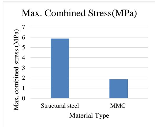
Fig. 9 Max. combined stress comparison
