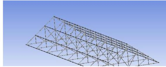
Figure 3: Discretized Model of Truss
