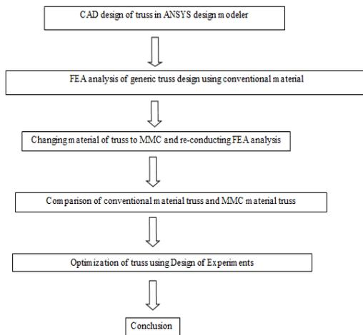
Fig. 1 Workflow for Truss Optimization Using Finite Element Analysis (FEA) and Material Modification
