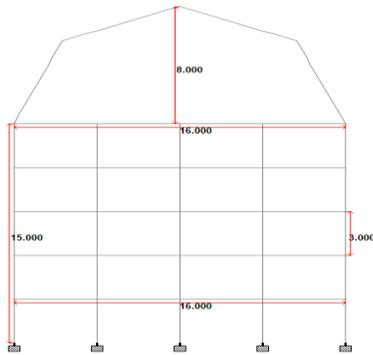
Figure 3 Detailing of the Curved roof building
