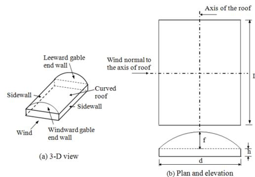
Figure 1 Schematic diagram of a curved roof at elevated level
